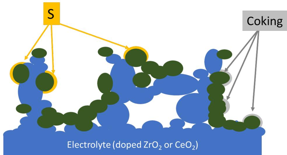
Sulphur tolerant and redox stable electrode materials
